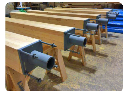
Brock Commons Tallwood House - Steel Connectors. Credit: Acton Ostry Architects ( flickr.com )
